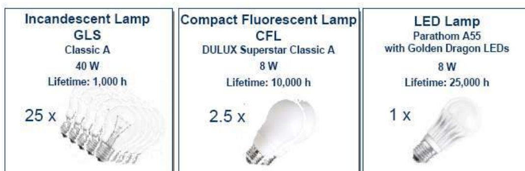
Figure 2: Type of lamps compared in the Life Cycle Assessment: a 40 W incandescent lamp, a compact fluorescent DULUX Superstar and a Parathom LED lamp
